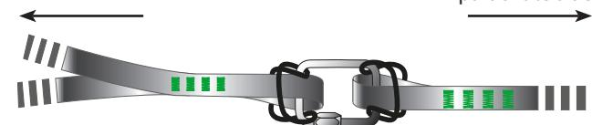
2. Connect the riser split side to the harness's shoulder attachment points using the provided stainless steel (Inox) 6 or 7 mm.
