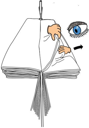
9. S-fold the left side of the canopy under the centre of the parachute, then S-fold the right side of the canopy onto the centre of the chute. Keep the canopy neatly folded in place using sandbags or books.
