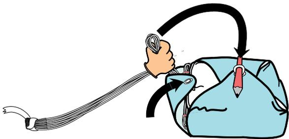
16. «S» fold the coil the remainder of the lines on the outside of the reserve parachute container.
