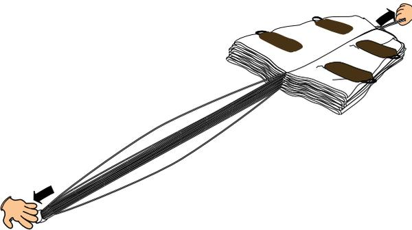
**2.** Keep the parachute unruffled with the lines running freely from the bridle «loop to loop» connection to the canopy's leading edge.
