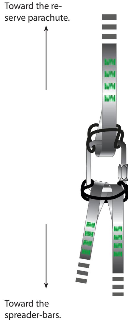
2. Connect the risers on top of each spreader bar (at the main loop), with the rectangular stainless steel maillons and the flexible elastic rings.
