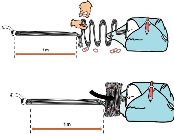
15. Close the fourth flap and insert about 4 cm of folded lines through the elasticated loop to keep the container closed.
