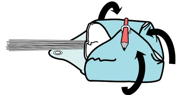
14. «S» fold the lines into the accommodating space left for them, leaving about 1m length of lines outside for the outer coils.
