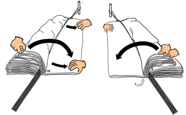
**6.** Be certain to have an equal panel ( gore ) count on each side ( the panel numbers may vary with other parachute models ). Be precise and verify that the bottom of the skirt ( leading edge ) is perfectly aligned and tidied..
