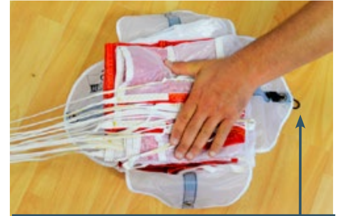
Position the POD's elastic loop opposed to the suspension lines.
