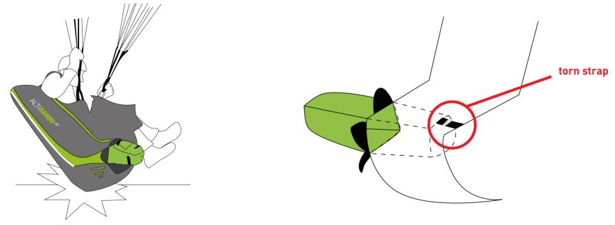
Our various tests show that the pocket damage does not take place when the reserve parachute is inside the rescue pocket (closed). The pocket could be damaged upon impact when used without housing the reserve parachute or when the emergency parachute is deployed.
