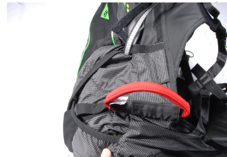
Handle positioning in its holding sleeve.
