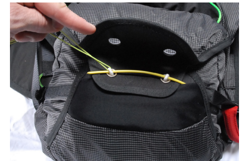
Push the loop through the upper flap grommet and push the yellow cable through it ( loop ).
