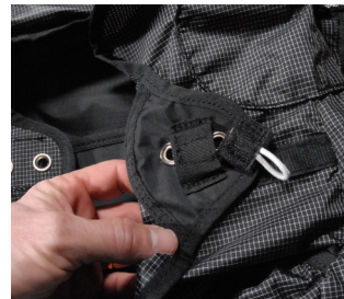
Pull on the rear flap, remove the cord from its grommet.
