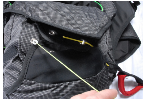
Push the cord through the left loop.
