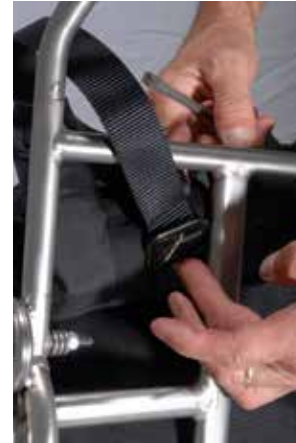
Wrap the strap around the frame and push it through the first buckle opening, and then through the second.
