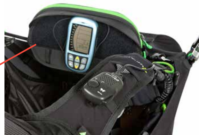
3 Cockpit with removable instrument support.
