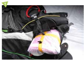
1 / Insert the reserve parachute inside the harness parachute pocket by opening all the flaps. The POD must be positioned with the handle at the top with risers and lines at the bottom. Push the risers through the guiding sleeves ( the risers must be located behind the parachute ).
