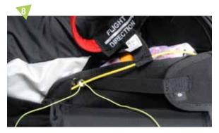
Push the handle's yellow cable ( rear section ) through the elasticated line and delicately remove the cord.
