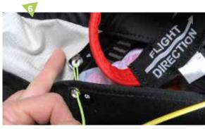
Push the end of the cord through the elasticated loop #4, then guide it through the grommets #5 and #6
