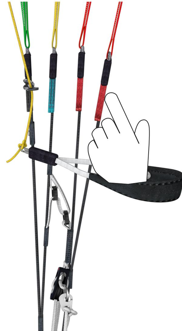
To reopen the "Ears", bring the accelerator/speedbar back to its neutral default setting, then let go the risers symmetrically. You can pump the brake handles on either side of the wing to facilitate its reopening sequence.
