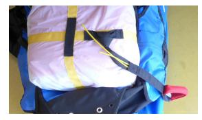
Insert the reserve parachute inside the harness parachute pocket by opening all the flaps. The POD must be positioned with the handle at the top with risers and lines at the bottom. Push the risers through the guiding sleeves ( the risers must be located behind the parachute ).
