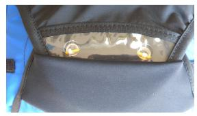
The yellow cable locks the reserve parachute pocket flaps in place. Tuck the upper flap inside its lower stretchable pocket. Check before every fligth for the yellow cable to be properly inserted through the two loops keeping the reserve parachute pocket securely
